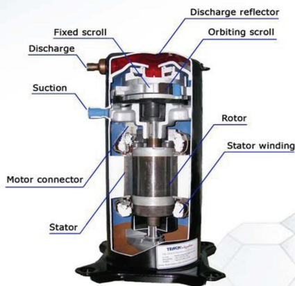
SECTIONED COPELAND SCROLL COMPRESSOR
